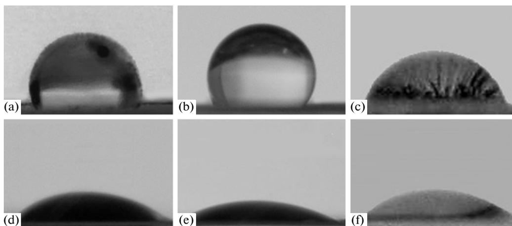
**Fig. 1.** Examples of typical contact angles of the CNM surface: SWNT-3 (a), NF (b), C60 (c), SWNT-2 (d), fNF (e), and C60(OH)<sub>-24</sub> (f).
