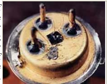
The first Mosfet transistor, designed by M. M. Atalla, D. Kahng, and E. Labate in late 1959. Courtesy: Lucent.
